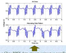
1.3 Gbps BPSK data stream using two parallel PCM implementations with 180° inversion
