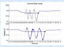
Scaling a sub-pulse with 8 possible "coarse" settings Analog controls allow fine adjustments (not shown)
