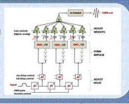
Chip contains 2 PCM modules and a memory block for storing 2 pulse shapes.
