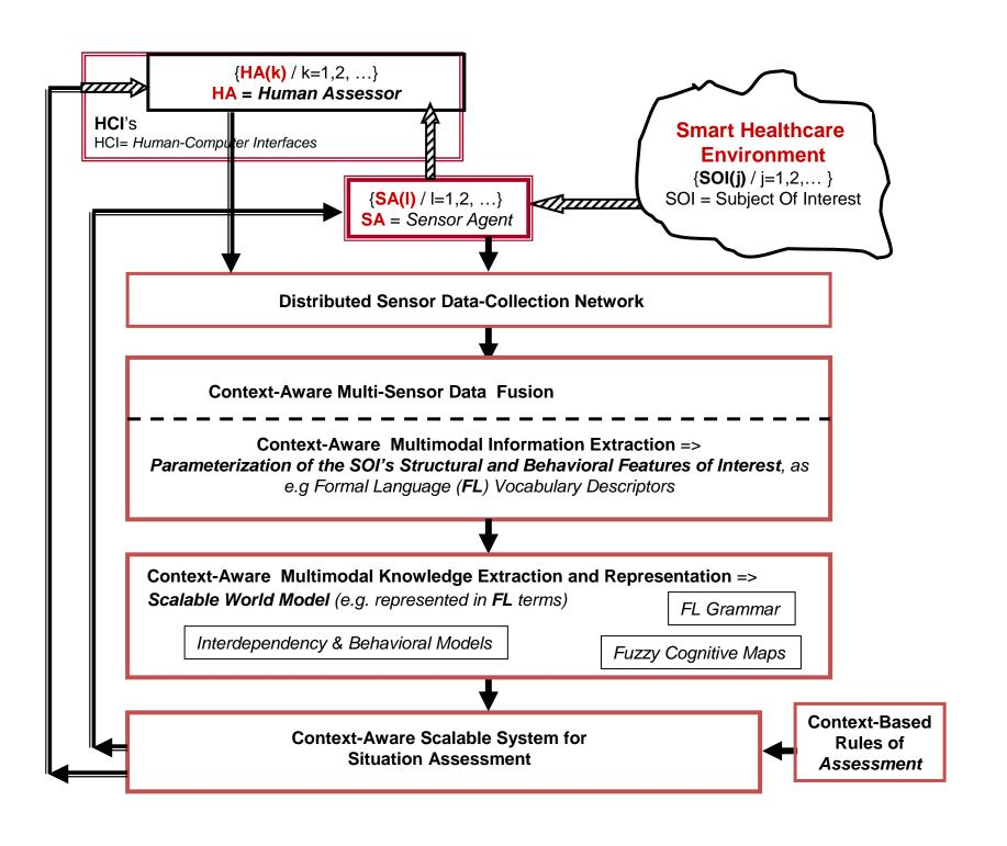
The **multi-sensor fusion architecture** is based on the **mission-critical JDL Data Fusion Model** developed by the Joint Directors of Laboratories Data Fusion Group .
