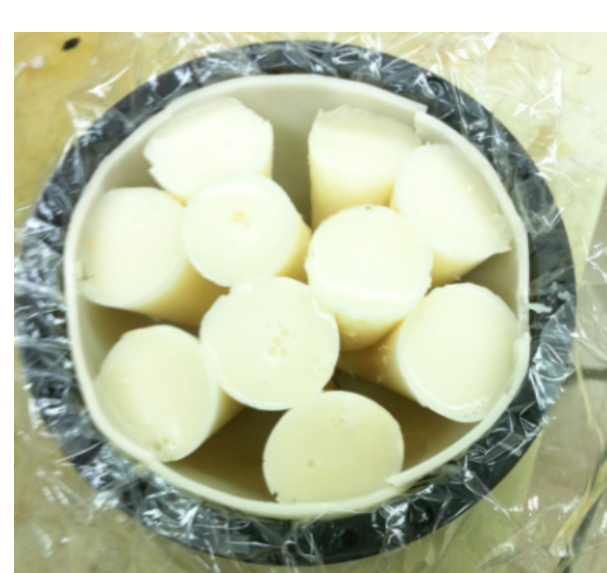
Fig.2: Photograph of Breast Phantom with conical glandular structures (70% by volume)
