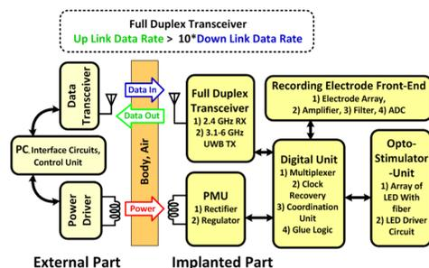
Fig. 2. General block diagram of proposed brain machine interface.
