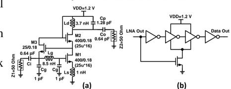
Figure 12: The circuit level of proposed LNA and Mixer as a receiver front-end.
