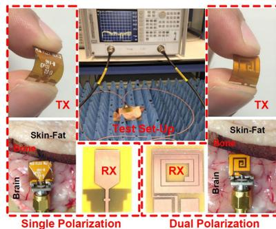
Fig. 6. Test setup for measuring the S-parameter of the single and dual polarization antennas.
