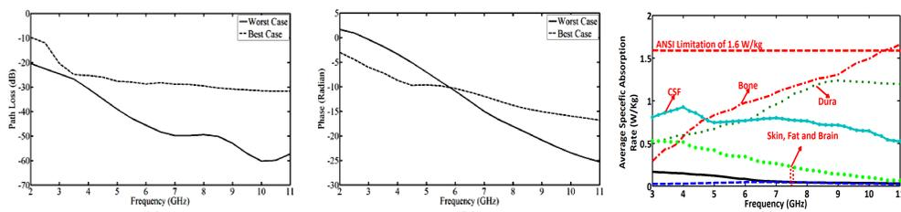
Fig. 7. a) Amplitude of the channel, b) phase of the channel, and c) simulated ASAR for different tissues.
