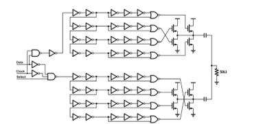
Fig. 11: The UWB transmitter circuit level structure.
