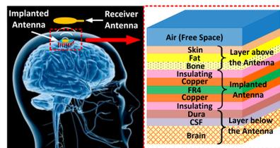
Fig. 5. Multi-layer model of the tissues for the parietal lobe region of the human head used for simulating channel behavior.
