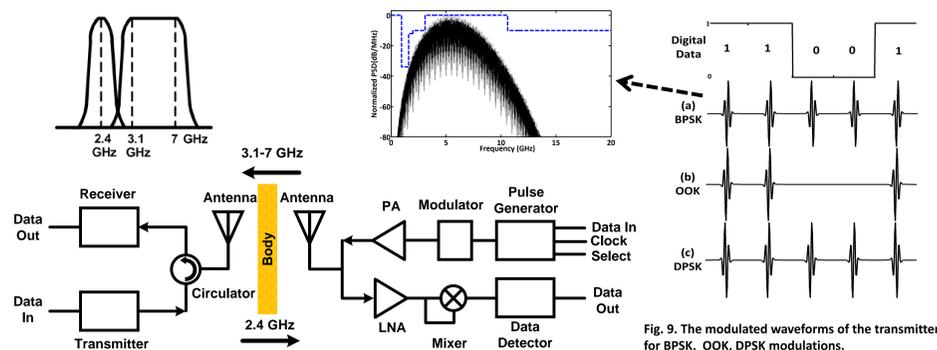
Fig. 8. The block diagram of the proposed full duplex transceiver.
