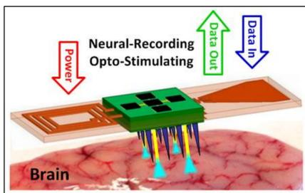
Fig. 4. The schematic of proposed neural recording and stimulating system (implanted side).
