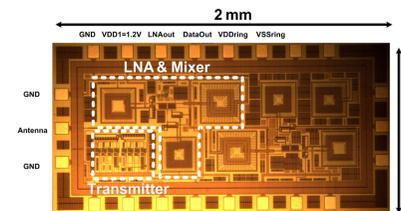
Figure 13: The chip micrograph (TSMC 180nm CMOS technology) of the proposed full duplex transceiver (0.5 mm<sup>2</sup>).
