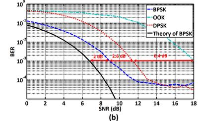
Fig. 10. The BER performances of the three modulations with different data rates a) 500 Mb/s and b) 2 Gb/s.
