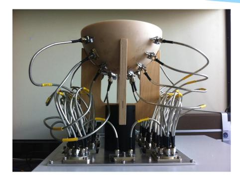
Travelling Wave Tapered and Loaded Transmission Line Antenna (Kanj 2008) Radiation efficiency = 39% Signal fidelity = 0.95
