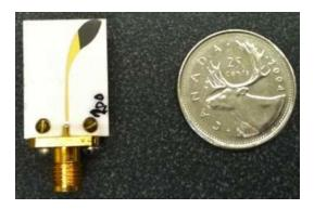
Designed for biosensing applications 0.635 x 12 x 15.8 mm<sup>3</sup> 11
